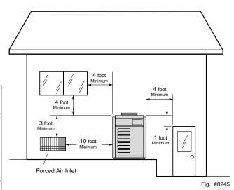
The point from where the flue products exit the heater must be a minimum of four (4) feet below, four (4) feet horizontally from or one (1) foot above any door, window or gravity inlet to a building. The top surface of the heater shall be at least three (3) feet above any forced air inlet, or intake ducts located within ten (10) feet horizontally.
